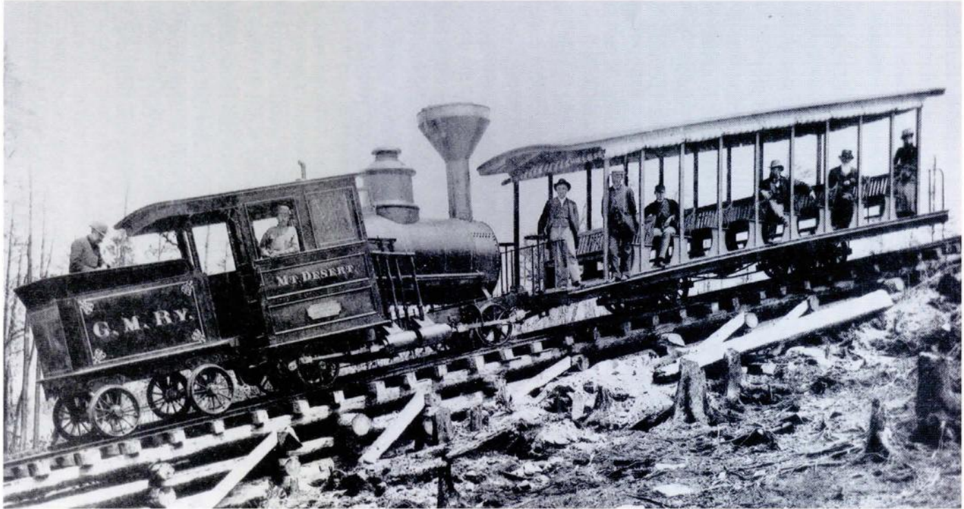
Green Mountain Railway locomotive No. 1, also called Mount Desert made the 1.2 mile journey between Eagle Lake and Green Mountains's central summit in slightly less than 30 minutes - an average speed of between two and three miles per hour.
