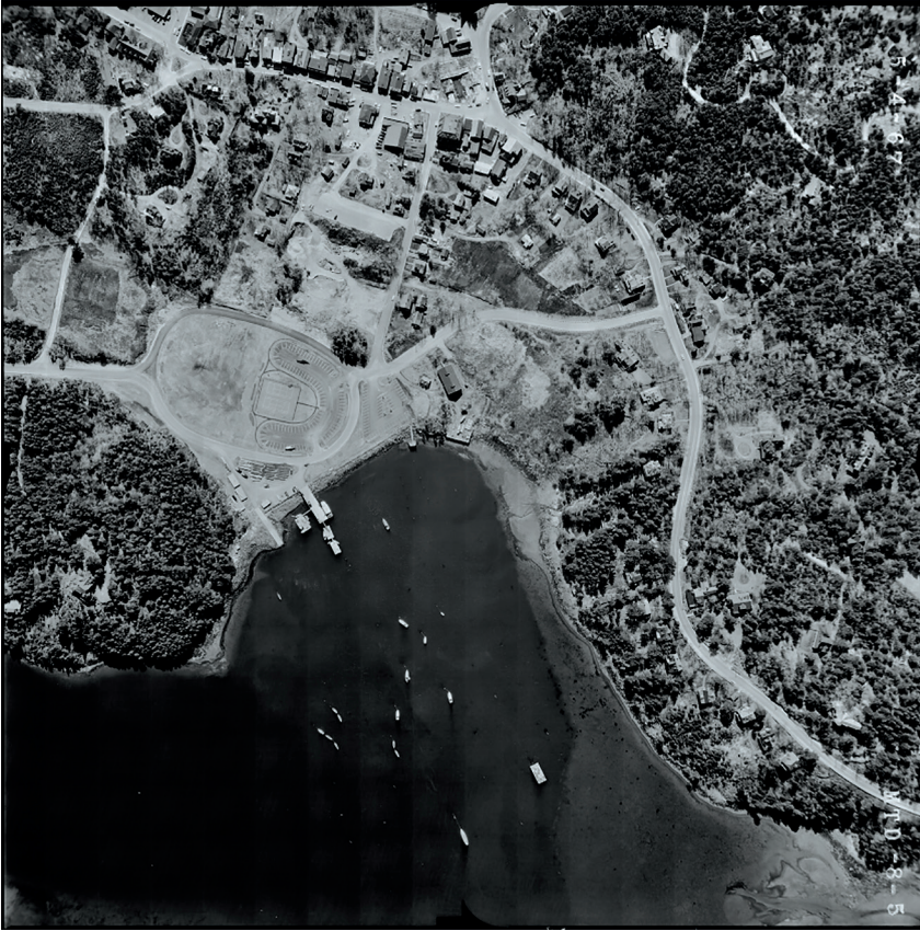
Silt and rock dredged from the harbor was pumped in behind the bulkhead to form the land used for today's marina. Courtesy of James W. Sewall Company
